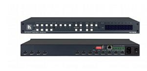
VS48H2 is a highperformance 4x8 matrix switcher for 4K@60Hz (4:4:4) HDR signals and digital audio routing. It reclocks and equalizes the signals and can route any one of 4 HDMI, HDCPcompliant sources (selectable) to any or all outputs simultaneously. VS48H2 offers unmatched audio flexibility where any embedded digital audio input can be routed to any digital output in addition to eight ARC sources to produce an equivalent 12x10 audio matrix
