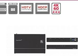
The VM-3H2 is a 1:3 distribution amplifier for up to 4K@60Hz (4:4:4) HDMI 2.0 signals, complying with HDCP 2.2 content protection standard. The unit takes one HDMI input, equalizes and reclocks the signal and distributes it to three identical outputs.
