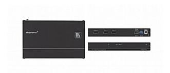
The VM-2H2 is a 1:2 distribution amplifier for up to 4K@60Hz (4:4:4) HDMI 2.0 signals, complying with HDCP 2.2 content protection standard. The unit takes one HDMI input, equalizes and reclocks the signal and distributes it to two identical outputs.
