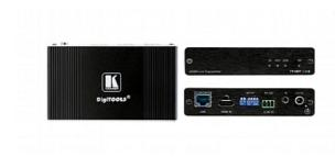
TP-583T is a high-performance, long-reach HDBaseT transmitter for 4K HDR HDMI, RS-232 and IR signals over twisted pair. TP-583T converts all input signals into the transmitted HDBaseT signal. It extends video signals to up to 70m (230ft) over Kramer copper cables at up to 4K@60Hz (4:4:4) video resolutions. It is compatible with standard HDBaseT-compliant extenders at 4K@30Hz and HD video resolutions
