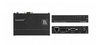
The TP-580R isa 4K UHD, twisted pair receiver for HDMI, bidirectional RS-232 and IR signals. It supports resolutions up to 4K@60 UHD (4:2:0). The TP-580T converts HDMI, RS-232, and IR signals into a twisted pair signal that it transmits to a TP-580R receiver. The TP-580R converts the twisted pair signal back into HDMI, bidirectional RS-232 and IR signals.
