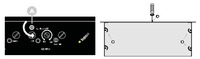
Unfasten screw (A) with a torx-screwdriver (see illustration). Now remove the 4 torx-screws (B) from the top lid. The top cover can be removed now. Gently lift the frontside a little, and slowly shift the lop lid to the rear. The connectorboard will become visible.
