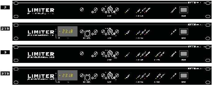
The SPL2, SPL2TS, SPL3 and SPL3TS are sound pressure limiters (SPL), especially designed for use in public houses, discotheques, etc. The SPL-limiters are no peak-limiters, they only limit the average sound pressure. Trimmers for on-site calibration are positioned behind removable cover(plates) which can be put under seal.
