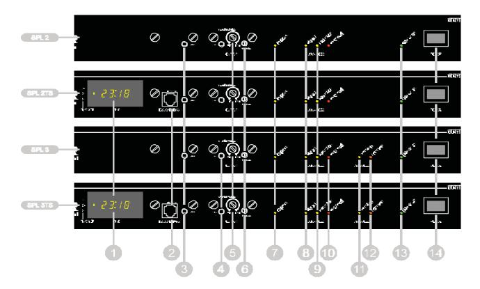
TIME display. In normal mode the LED-display shows the time-of-day, in military format (24h-format). When switching on the limiter, the date and time will scroll
