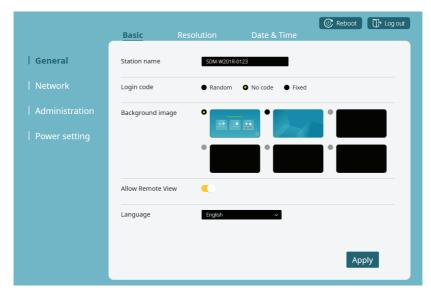
1) **Station Name:** The module's display name is shown on the standby screen and the Hyshare Pro app's station list. It will also be used as the SSID (Wi-Fi name) for the wireless access point.
