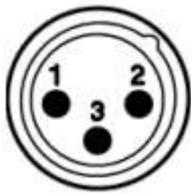
Pin 1: Masse Pin 2: Signal + Pin 3: Signal -
