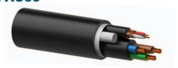
The PAC60 is a high quality DMX-AES and power cable in one jacket. The cable consists of a power cable and a DMX-AES signal cable. A general outer jacket with an O.D. of 17 mm made of flexible PVC protects each inner cable against abrasion. The CE - VDE approved inner power cable contains 3 conductors with a section of 2,5 mm², protected by a PVC jacket with an outer diameter of 9 mm.
