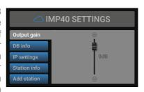
or counter-clockwise (tuning down). Press the rotary dial for confirming the currently set output level.
