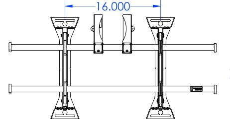
COMPONENT DIMENSION LIMITS WHEN INSTALLED IN MIDDLE OF UPPER BAR MAX WIDTH = STUD DISTANCE - 6.25" MAX HEIGHT = N/A
