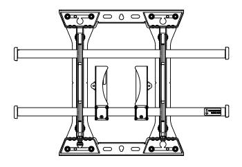
OPTIONAL SIDE POSITIONS FOR MEDIUM, LARGE AND XLARGE FUSION MOUNTS (MEDIUM SHOWN)
