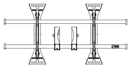
COMPONENT DIMENSION LIMITS WHEN INSTALLED IN MIDDLE OF BOTTOM BAR MAX WIDTH = STUD DISTANCE - 2.50" MAX HEIGHT = 4.75"
