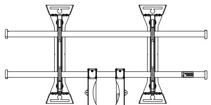
COMPONENT DIMENSION LIMITS WHEN INSTALLED IN MIDDLE OF LOWER BAR MAX WIDTH = STUD DISTANCE - 6.25" MAX HEIGHT = N/A
