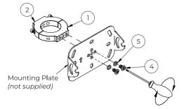
\*Important: Ensure to fix the mounting plate to the front half of the collar (item 1) so you have access to item 3 on the back.
