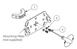
\*Important: Ensure to fix the mounting plate to the front half of the collar (item 1) so you have access to item 3 on the back.
