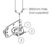
**Note:** Mounting plates can also be attached to the collar after the collar is fixed onto the pole.
