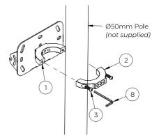
**Note:** Mounting plates can also be attached to the collar after the collar is fixed onto the pole.
