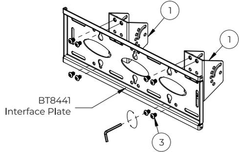
2. Using *items 2 & 3*, fix *item 1* to the Ø50mm collars that have been pre-assembled onto the Ø50mm poles.
