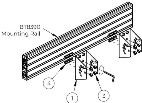
2. Using *items 2 & 3*, fix *item 1* to the Ø50mm collars that have been pre-assembled onto the Ø50mm poles.
