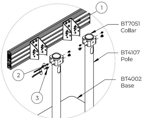
3. Set the required tilt angle by adjusting *item 1* and fix tilt in position using *item 3*.
