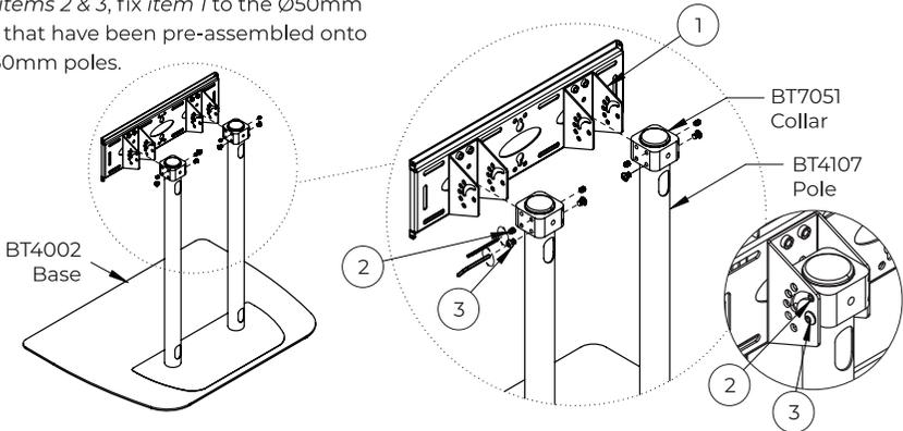
3. Set the required tilt angle by adjusting *item 1* and fix in position using *item 3*.
